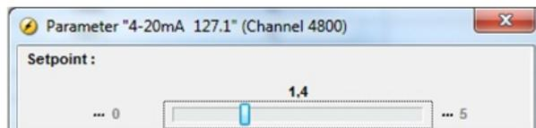
In the example shown above, the value can be adjusted with one decimal. If the parameters were not refreshed, it would still only be possible to adjust the set point without decimals.
